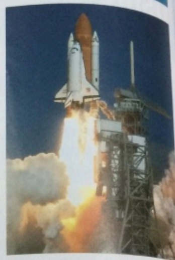
For lift-off the main engines burn hydrogen. Additional thrust comes from solid fuel in the white boosters.
