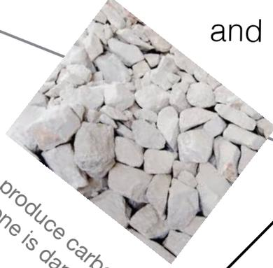
Limestone is heated with clay to make cement. Cement is mixed with sand and aggregate to make concrete.
