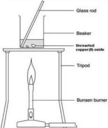
**b** When the acid is hot enough (just before it starts to boil), use a spatula to add small portions of copper(II) oxide to the beaker. Stir the mixture gently for up to half a minute after each addition.
